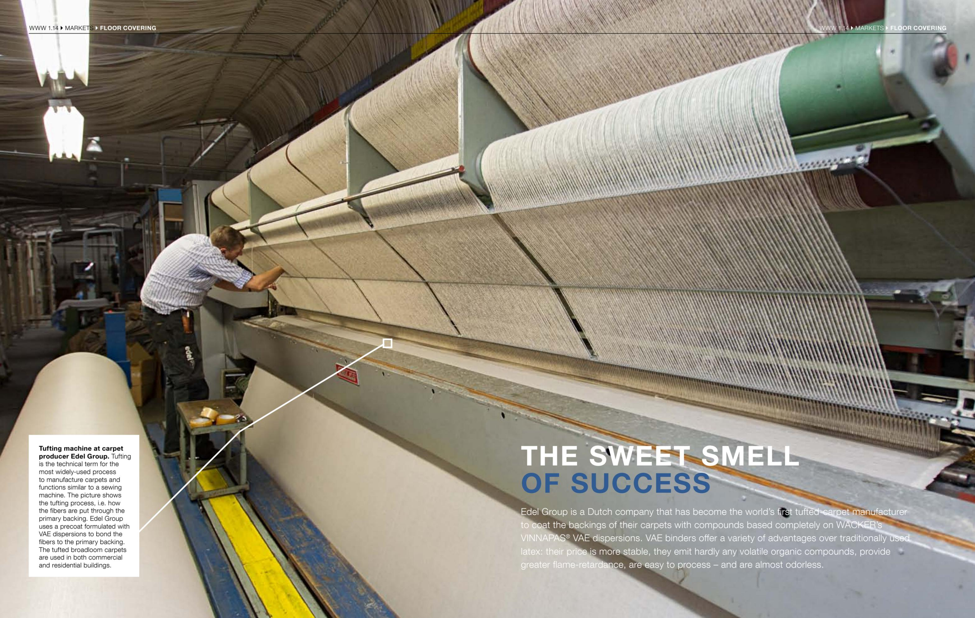
**Tufting machine at carpet producer Edel Group.** Tufting is the technical term for the most widely-used process to manufacture carpets and functions similar to a sewing machine. The picture shows the tufting process, i.e. how the fibers are put through the primary backing. Edel Group uses a precoat formulated with VAE dispersions to bond the fibers to the primary backing. The tufted broadloom carpets are used in both commercial and residential buildings.
