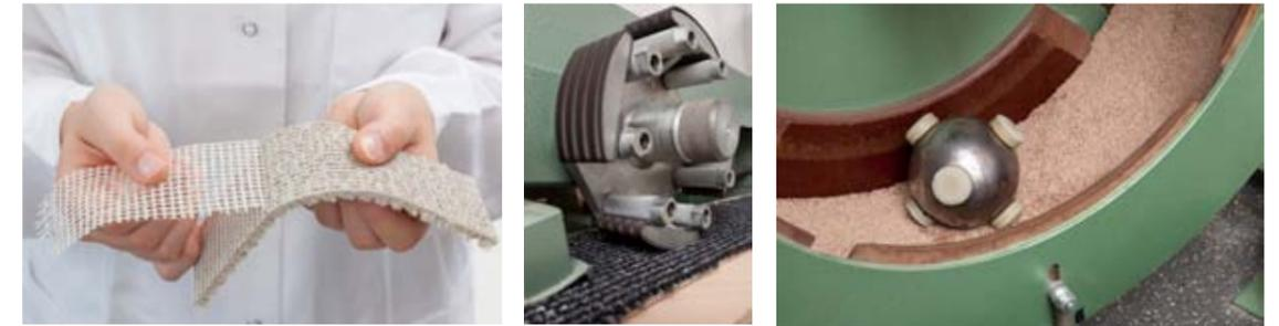
The delamination test, Lisson test and Vettermann drum test are three additional tests conducted at WACKER's carpet laboratory. The delamination test (left) evaluates the adhesion of the backing to the carpet. The Lisson test (center) and the Vettermann drum test (right) are used to simulate the daily stress a carpet is submitted to, such as through footsteps and rolling office chairs.
